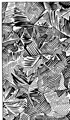
FIG. 2.—SPANGLES ON SURFACE OF GALVANIZED SHEET STEEL
